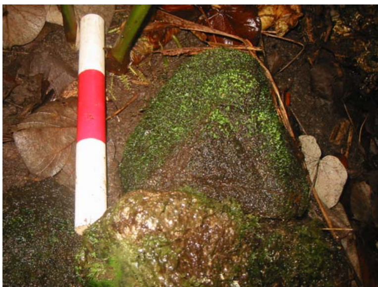
Figure 4. Survey control point engraved in stone and depicted on map (Podmore 1915). The scale is marked in 10 cm increments.
